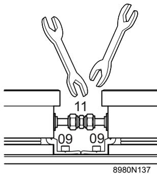
**i** The vertical play in the junction plate allows access to the hydraulic connections and makes it possible to secure the solar collectors.
