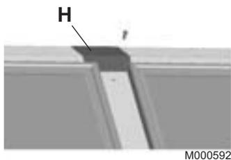
13. Secure the junction plate to the upper covering part using a self-tapping screw.
